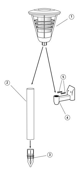
A flathead screwdriver is required for mounting the wall bracket.
